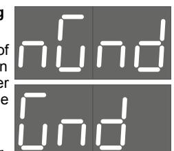
**Attention!** Operation of the heater without grounding is not allowed. This function is intended only for verification purposes of the device working capacity during the absence of the outlet with the grounding.
