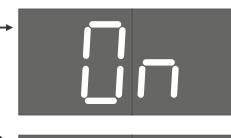
**4 Switching off and on of the heating.** Simultaneously press and hold both buttons (more than 2 seconds) until the corresponding indication and sound confirmation (see on the right) appears.
