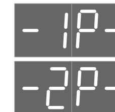
If you do not have enough power of the power grid (turns on the breaker box). You can turn on the automatic power reduction function of the heater (by 50%) when the set temperature is reached.
