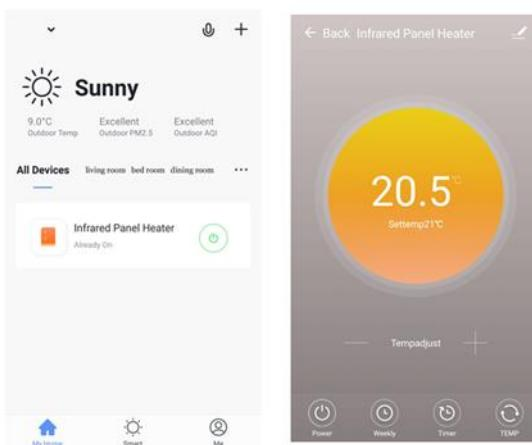
2. Click the green button to turn the heater power on or off. The blue indicator on the heater panel lights up, which means the heater is turned on.
