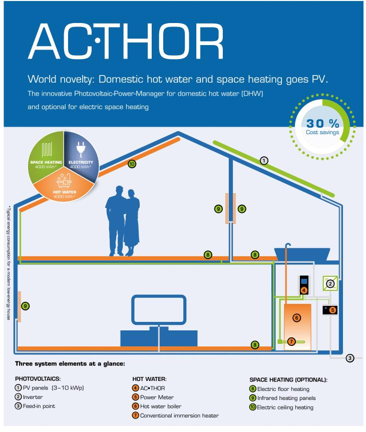
Electricity, hot water and optional electric heating from solar power: All this is possible with **AC•THOR** and **Power Meter**. This enables entire electrical building installation: cables instead of pipes. Simple and economical! The power meter detects the power flows of the PV system and transmits data to the AC•THOR. Excess energy is used for heat generation (primarily hot water, secondarily space heating).
